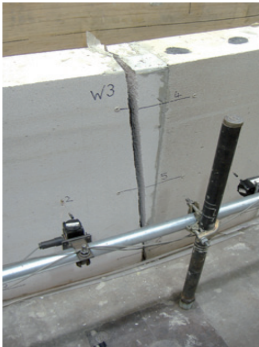
Fig. 3. Failure of Wall 3 under Horizontal Spanning, Note the Unit Failure and not Mortar Joint Failure.
